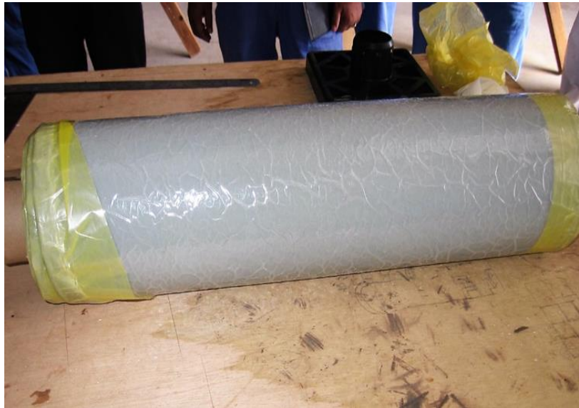
A roll of uncured GRP must be protected from light and moisture until fully cured.
