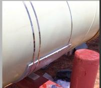
ProClad Wearpads are a minimum thickness of 5mm and are manufactured specifically to the diameter size of the pipes for which they are intended. The standard Wearpad is made for a 120° degree sizing and have a standard length of 12 inches.
