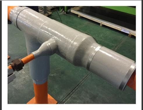
ProClad is delivered as pre-molded parts for straights, fittings, end caps, flange boxes and valve boxes. ProClad pieces are joined with ProClad's range of exclusive adhesives. The ProClad system is designed to encapsulate the entire insulation system End cap to End Cap
